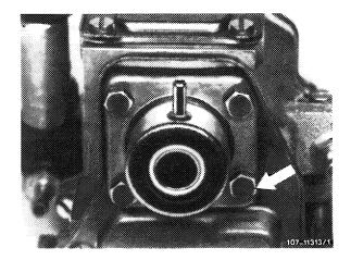
2 Check position of control rod. Push guide lever on cylinder head cover to stop while measuring position of control rod. For this purpose, insert plug gauge through bore against control rod and mark position of plug gauge.
