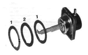
1 Gasket 2 Steel ring 5 To make sure, subsequently check control rod position once again as described in item 2. The mark on plug gauge should again be in alignment.
